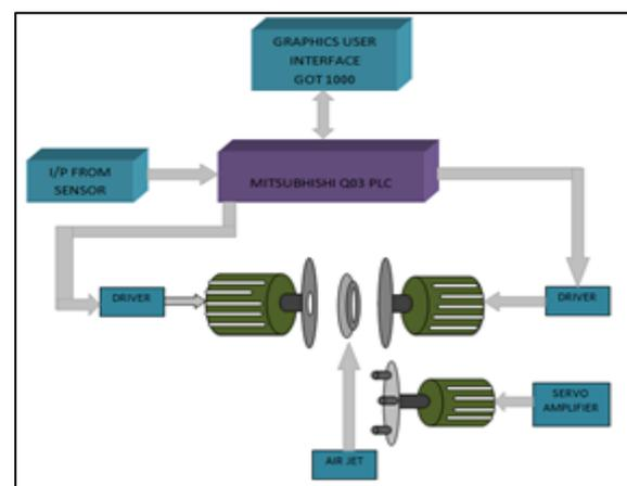
Fig. 2: Block Diagram of the integrated PLC
