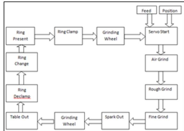
Fig. 1: Work sequence of DG300 Grinding Machine
