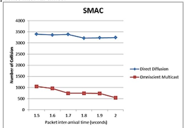
Fig. 4.3: Collision Counts V/S Packet Inter-Arrival Time.
