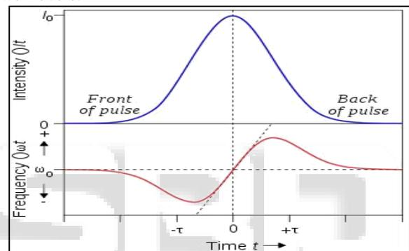
Fig. 1: A pulse (top curve) propagating through a nonlinear medium undergoes a self-frequency shift (bottom curve) due to self-phase modulation.
