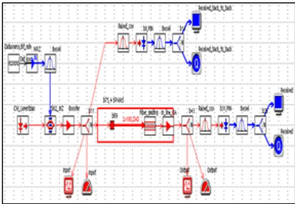
Fig. 2: Simulation Setup for Self Phase Modulation Using OPTSIM
