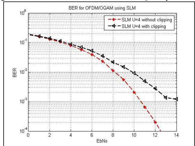
Fig. 6: BER Vs. Ebno of Conventional SLM ( $U=4$ ), SLM With Clipping.
