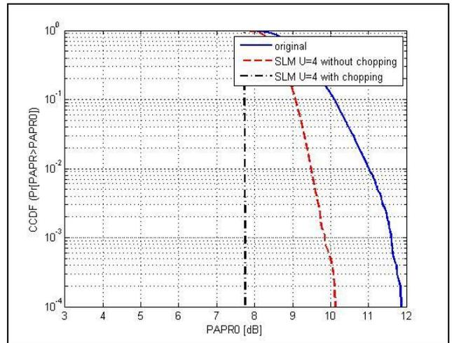
Fig. 5: CCDF vs. PAPR for SLM with clipping and conventional SLM with  $U=4, 16$ -QAM,  $N=1024$ .
