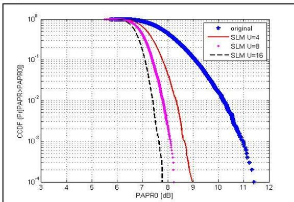
Fig. 4: CCDF Vs. PAPR For Conventional SLM With Different U, 16-QAM, N = 1024.
