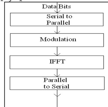
Fig. 1: Typical OFDM Transmitter
