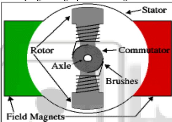
Fig. 2: Pole DC Motor
