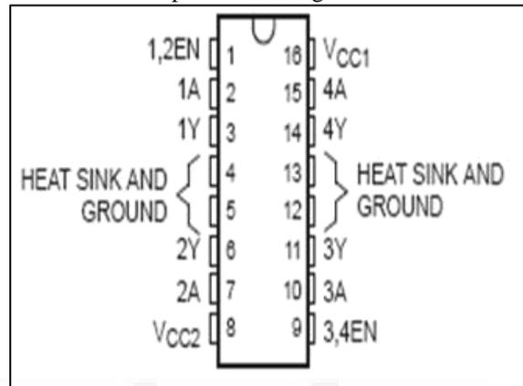
Fig. 3: Pin Diagram of L293D
