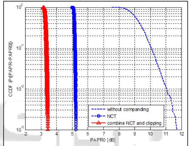
Fig. 3: PAPR reduction performance for case (3)  $c = 0.001$ ,  $k_2 = -0.20$  with  $N = 1024$ , QPSK modulation and oversampling factor  $L = 4$ .
