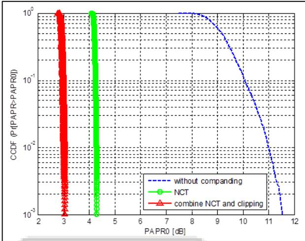
Fig. 1: PAPR reduction performance for case (1)  $c = 0.25$ ,  $k_2 = -0.001$  with  $N = 1024$ , QPSK modulation and oversampling factor  $L = 4$ .
