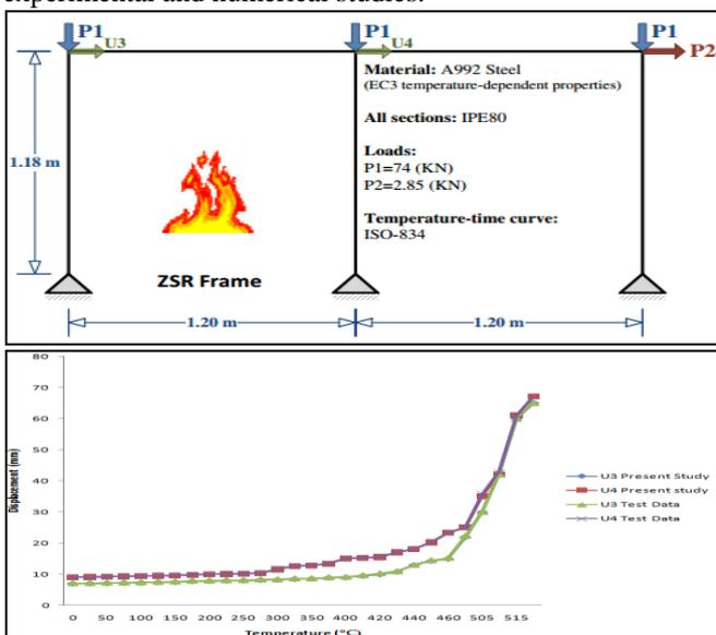
Fig. 2: ZSR Steel Frames Used In the Validation Analysis and Their Corresponding Results
