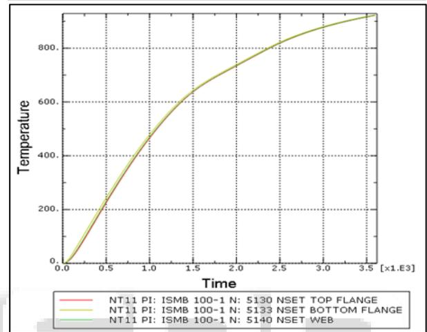
Fig. 6: Time-Temperature Curve in Frame without and With Radius Cut RBS
