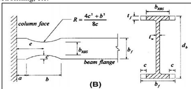
Fig. 1: Reduced Beam Section Connection Detail
