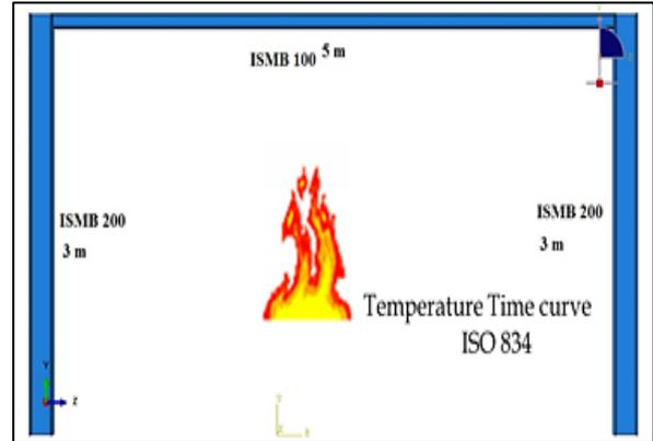
Fig. 3: Steel Frames with Fire Case
