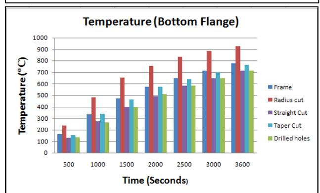
Fig. 7: Comparison of Results in Frame Without and With Different Pattern of RBS
