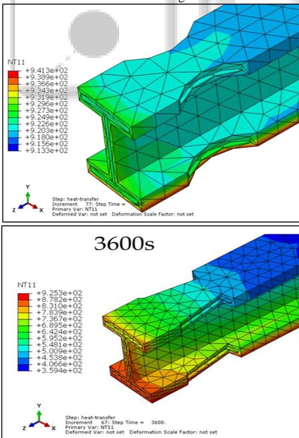
Fig. 5: Temperature Distribution in Frame with Radius Cut and Taper Cut RBS
