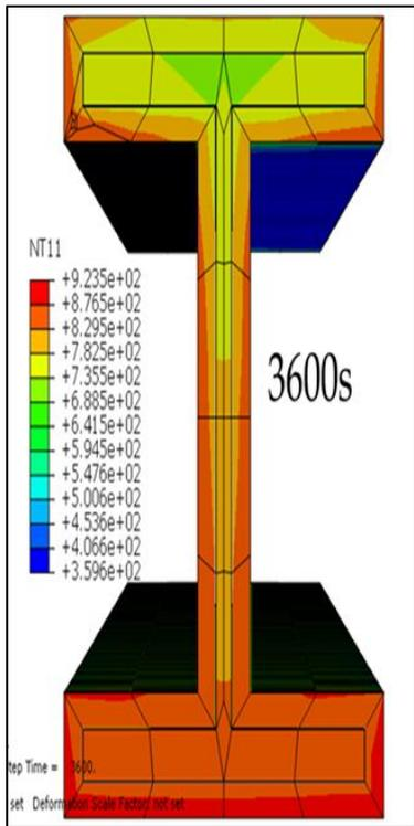
Fig. 4: Temperature Distribution in Steel Frame without RBS
