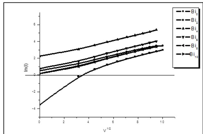
Fig. 3: Verification of Poole Frankel conduction mechanism
