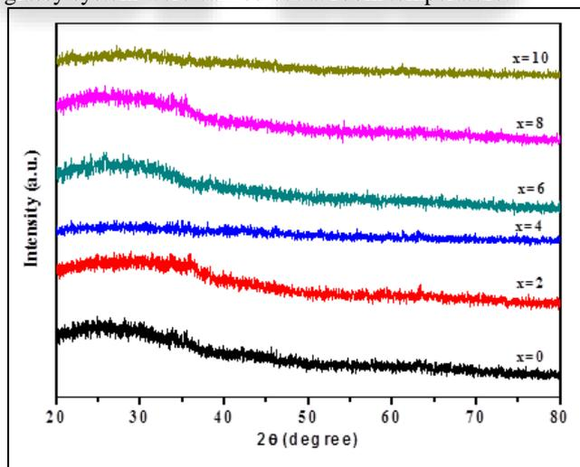
Fig. 1: XRD pattern of  $\text{Se}_{90-x}\text{Sb}_{10}\text{Bi}_x$  (Where  $x=0, 2, 4, 6, 8, 10$ ) chalcogenides glasses at room temperature
