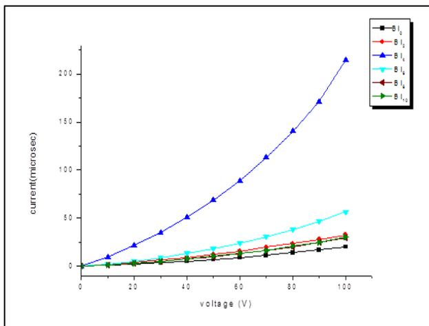
Fig. 2: I-V characteristics of Se<sub>90-x</sub>Sb<sub>10</sub>Bi<sub>x</sub> (Where x=0, 2, 4, 6, 8, 10) chalcogenides glasses at room temperature.
