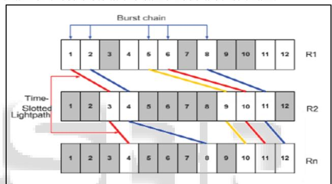
Fig. 2: Burst chain and time slotted light path
