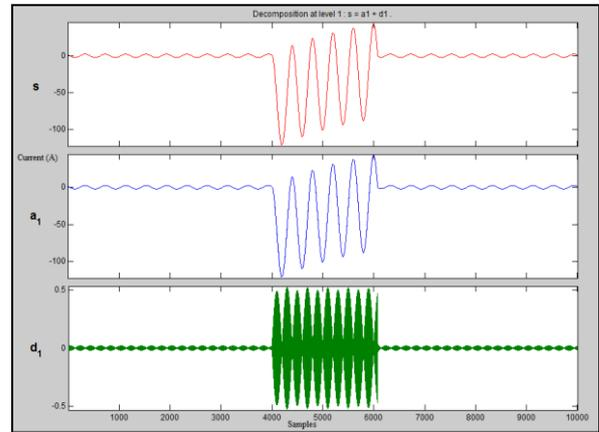
Fig. 5: First Level Decomposition of Phase 'A'
