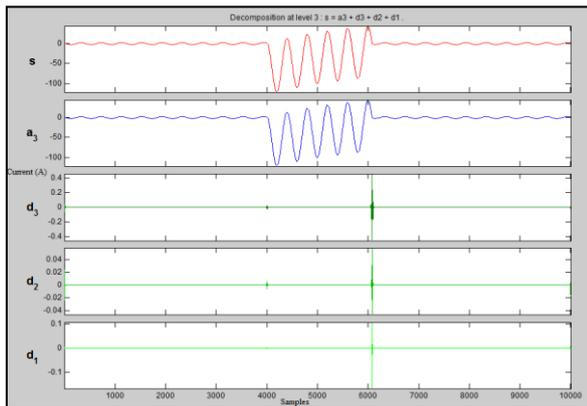
Fig. 8: Levels of Decomposition of Phase 'A'
