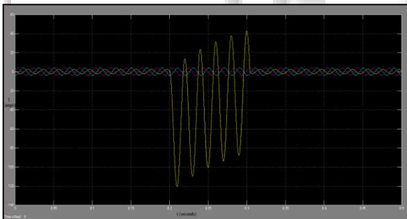
Fig. 4: Current Waveforms for an L-G Fault
