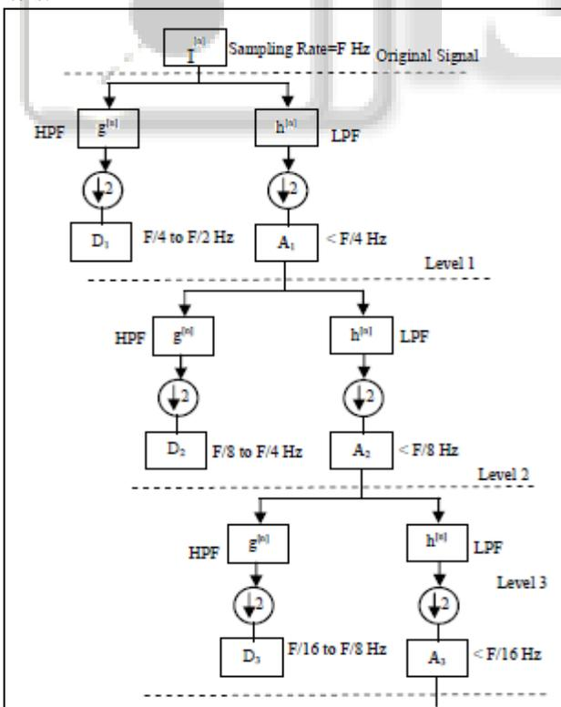
Fig. 1: Schematic Diagram of Multi-Resolution Analysis of DWT Decomposition
