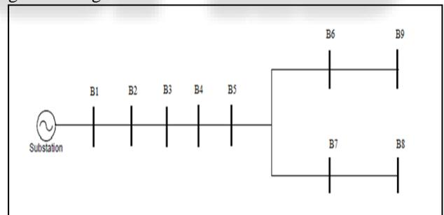
Fig. 2: Single Line Diagram of the 9-Bus Distribution System
