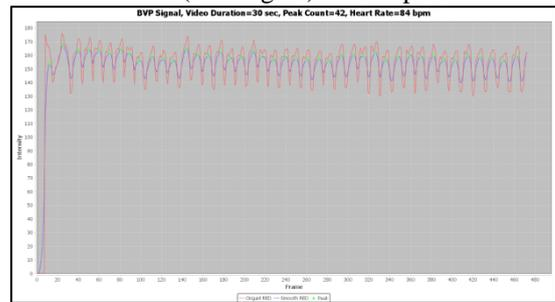
Fig. 9: Blood Volume Pulse Signal (Red Signal) And Peak (Green Triangles) Counting On Smoothed Blood Volume Pulse (Blue Signal) For Sample4
