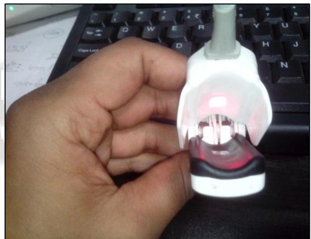
Fig. 2: Pule Oximeter Probe Attached To Philips Intellivue Multipara Monitor (Input)
