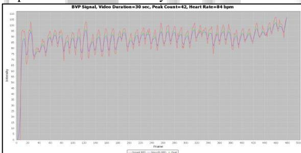
Fig. 6: Blood Volume Pulse Signal (Red Signal) And Peak (Green Triangles) Counting On Smoothed Blood Volume Pulse (Blue Signal) For Sample1
