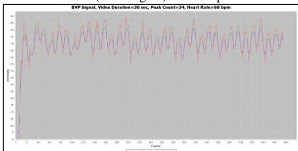
Fig. 7: Blood Volume Pulse Signal (Red Signal) And Peak (Green Triangles) Counting On Smoothed Blood Volume Pulse (Blue Signal) For Sample2
