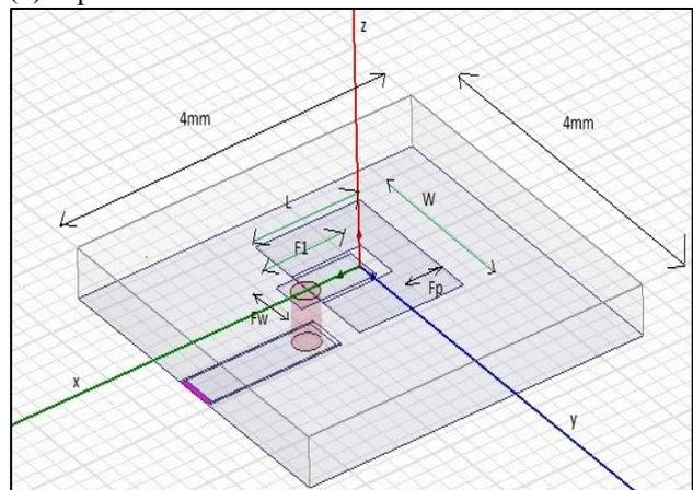
Fig. 1: Geomrtey of L-Probe Microstrip Antenna Element
