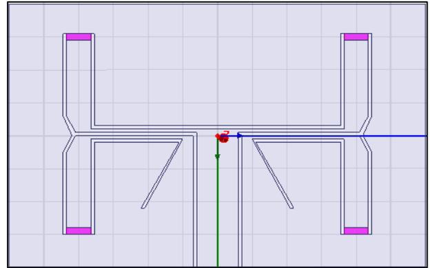
Fig. 3: Geometry of CPW Feed Network
