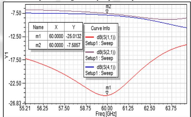
Fig. 4: Simulated Results of S-Parameters
