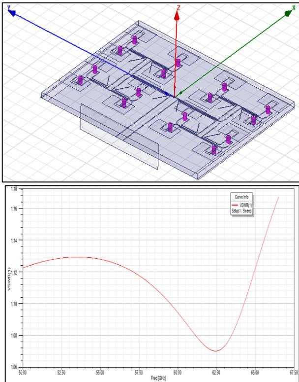
Fig. 6: VSWR Plot with the Frequency
