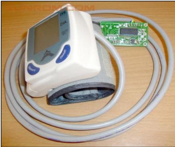
Fig. 3: Blood Pressure Module
