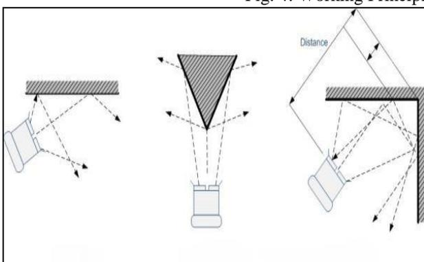
Fig. 5: Reflection of Sound through Various Surfaces
