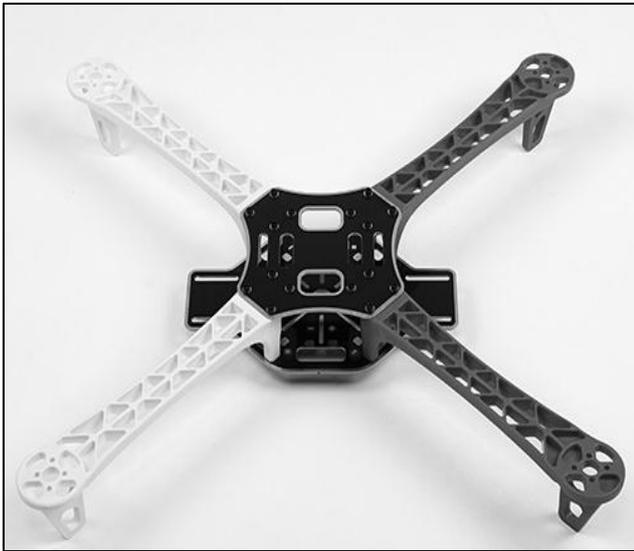
Fig. 1: Quadcopter Frame
