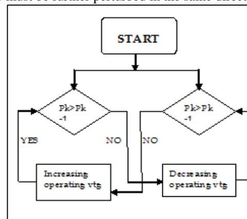
Fig. 3: Flowchart of Perturb and Observe Method
