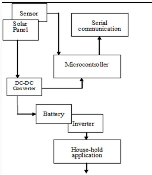
Fig. 1: Block Diagram of Solar Panel Using MPPT. The block diagram consists of following parts:-
