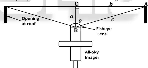
Fig. 1: Geometry Showing Determination of the Field Of View of All Sky Imager
