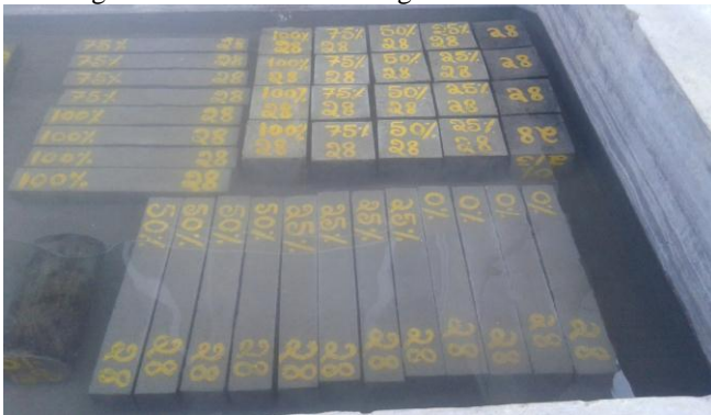
Fig. 2: Curing of 28 days specimens
