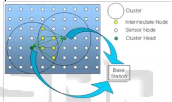
Fig. 3: Redundant data reported to Base Station caused by overlapped area
