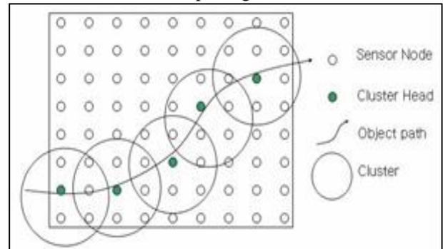
Fig. 1: Dynamic Clustering Mechanism for OTSN
