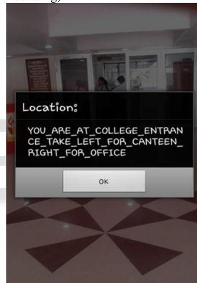
Fig. 5: Image Recognition mode showing the current location and directions to other locations by recognizing live video feed
