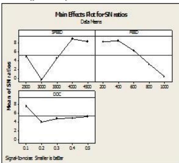
Fig. 1.2: S/N Ratio for Milling Parameter
