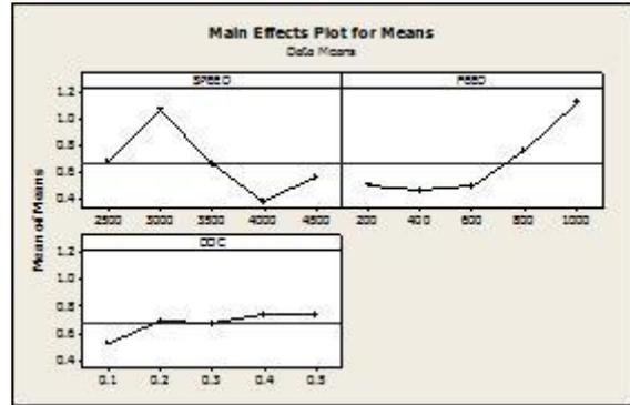
Fig. 1.3: Mean Plot for Milling Parameter
