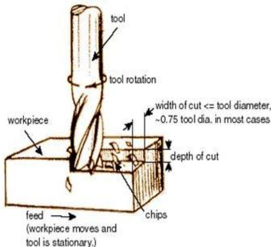
Fig. 1.1: Milling Operation
