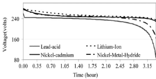
Fig. 4: Battery Voltage Versus Time Of Use, For A Range Of 240 V /100 Ah, Batteries At A Discharge Current Of 1.5 C/5 (30 A).
