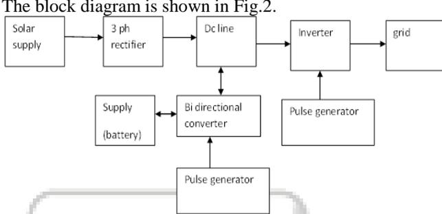
Fig. 2: Block Diagram of Grid Connected Eco Friendly
