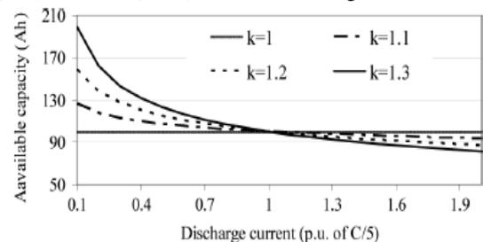
Fig. 3: Effective Battery Capacities At Different Discharge Currents, 100 Ah At 5h
