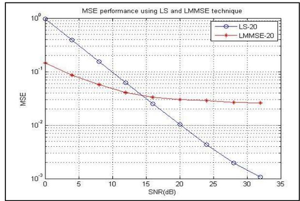
Fig. 6: MSE Vs SNR for L=20
