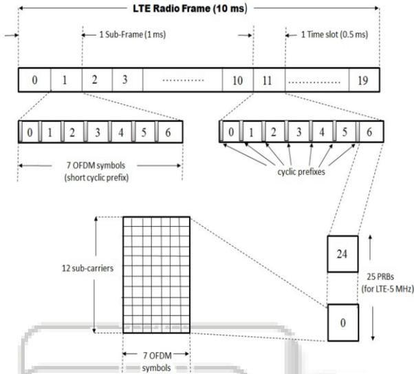
Fig. 1: LTE Radio Frame Structure[4]
