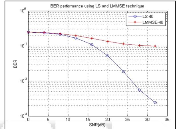
Fig. 7: BER Vs SNR for L=40
