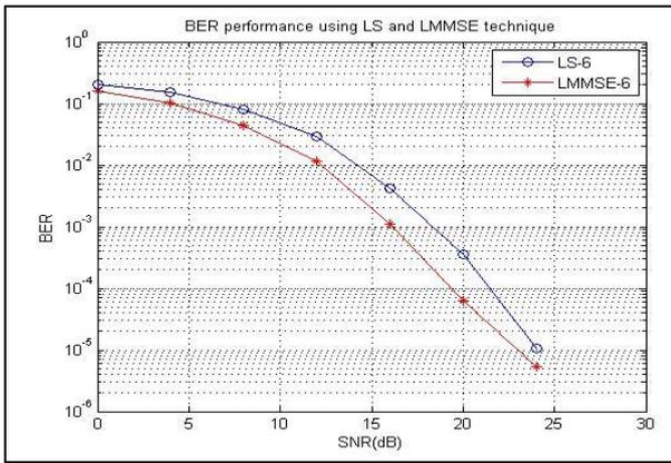
Fig. 3: BER Vs SNR For L=6
