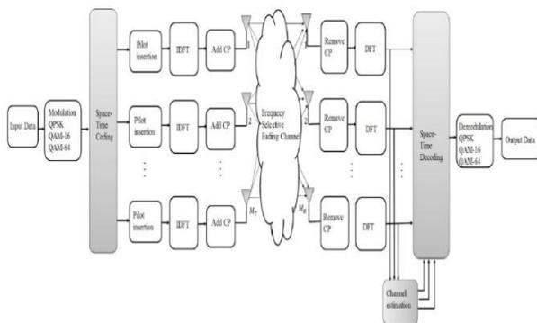
Fig. 2: LTE Downlink System Model[4]
