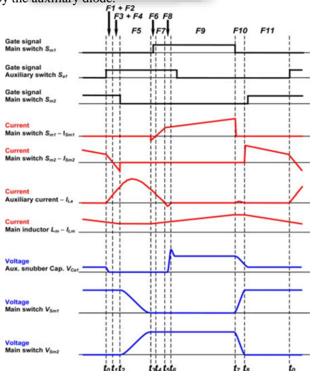
Fig. 5: Basic Wave Forms in the Forward Boost Operation
