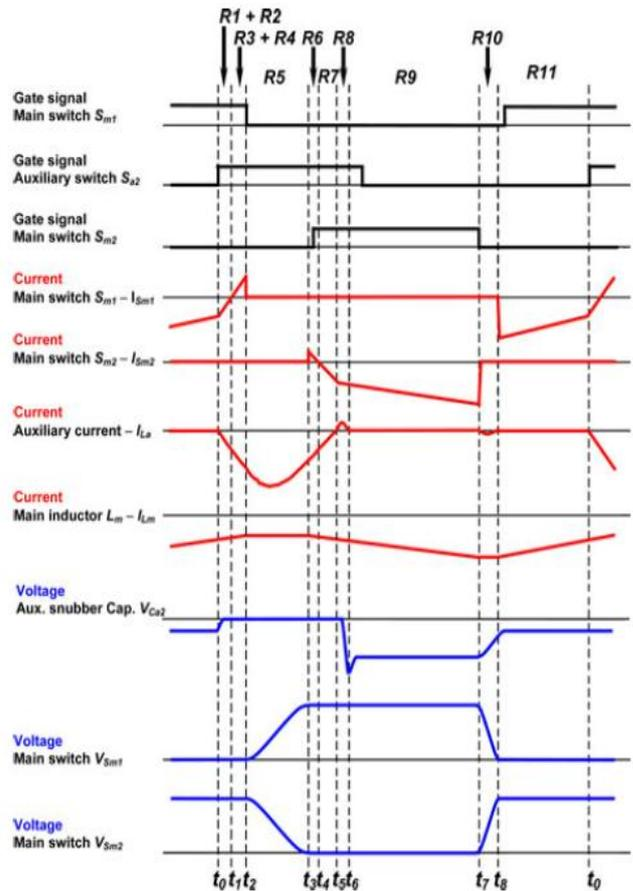
Fig. 6: Basic Wave Forms In The Reverse Buck Operation
