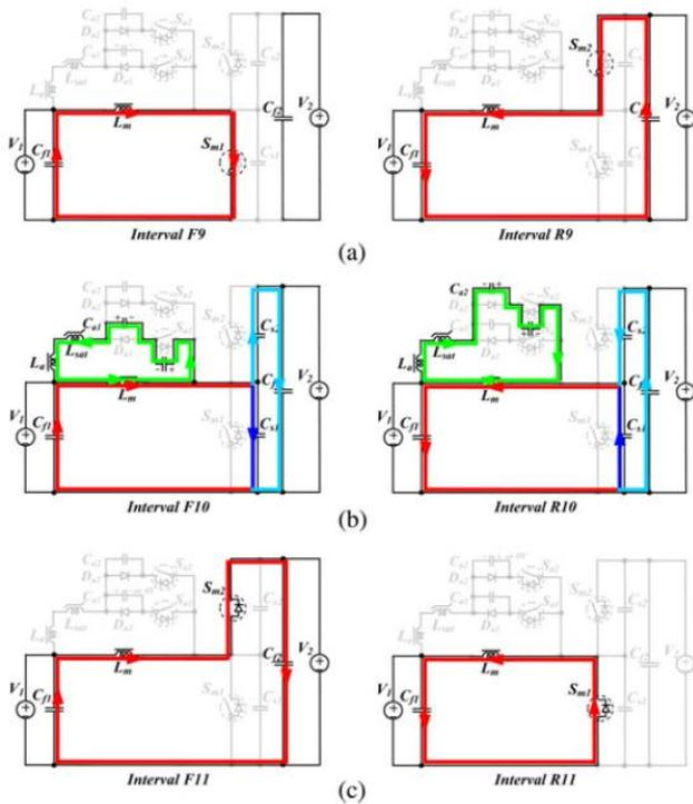
Fig. 7: Main Circuit Intervals In Boost And Buck Operation
