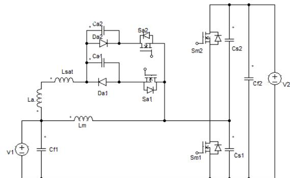
Fig. 4: Forward Boost Reverse Buck Dc-Dc Converter With Simple Snubber
