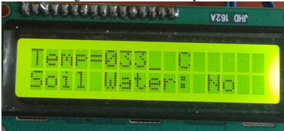
Fig. 6: Display of No Moisture In Soil
