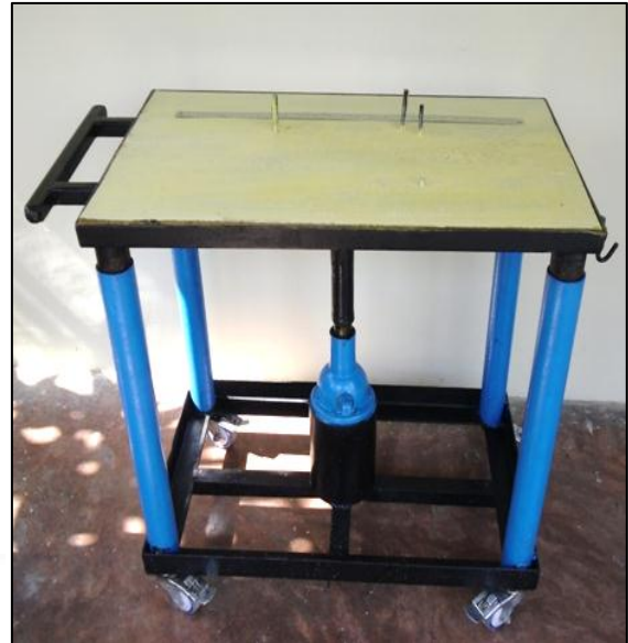
Fig. 1: Platform with Jig and Fixture with Height Adjustment and Provision for Marking and Measuring
