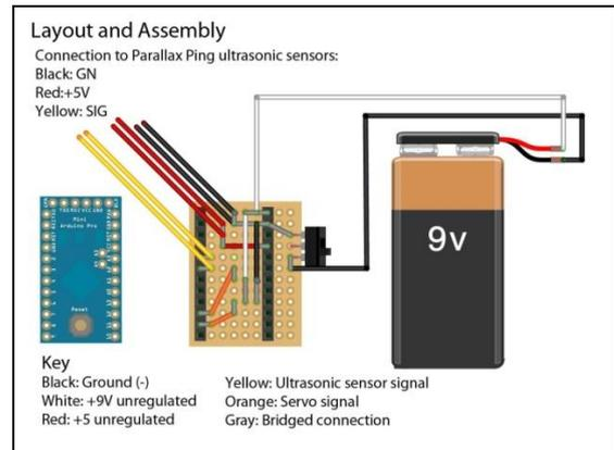
Fig. 4: Layout and Assembly
