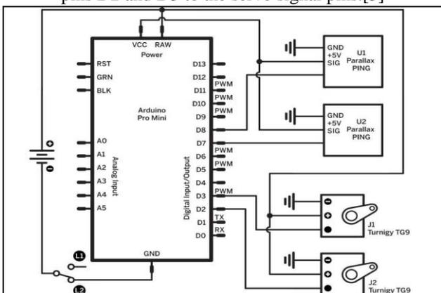
Fig. 3: Schematic Diagram of ST.R.O.N.G
