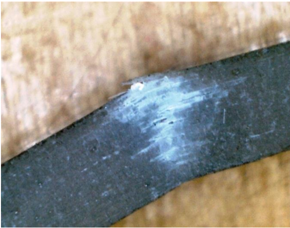
Fig. 19: Delamination effect on the Glass fiber
