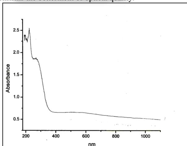
Fig. 5: UV-Vis-NIR Spectrum of Pure KDP Crystal
