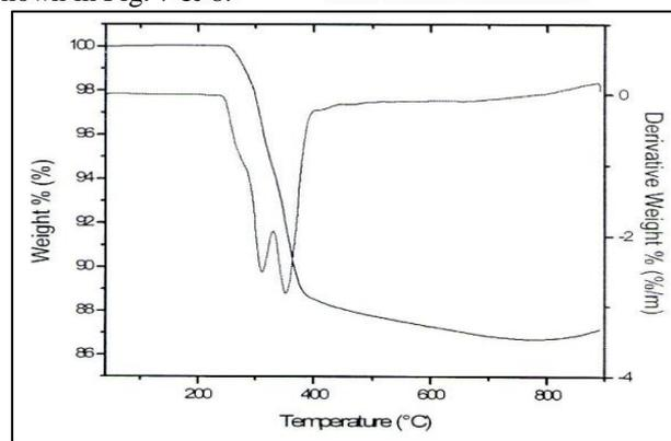
Fig. 7: TG/DTA Curve of Pure KDP Crystal
