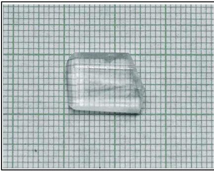
Fig. 2: Magnesium Chloride added KDP Crystal
