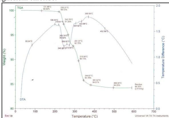
Fig. 8: Added KDP Crystal. TG/DTA Curve of Magnesium Chloride
