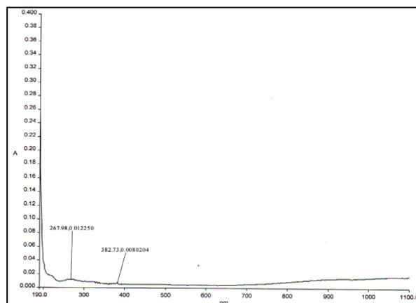
Fig. 6: UV-Vis-NIR Spectrum of Magnesium Chloride added KDP Crystal
