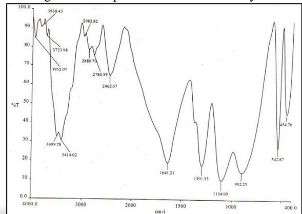
Fig. 4: FTIR Spectrum of Magnesium Chloride Added KDP Crystal
