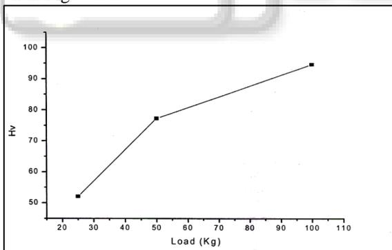
Fig. 9: Microhardness Curve of Pure KDP Crystal
