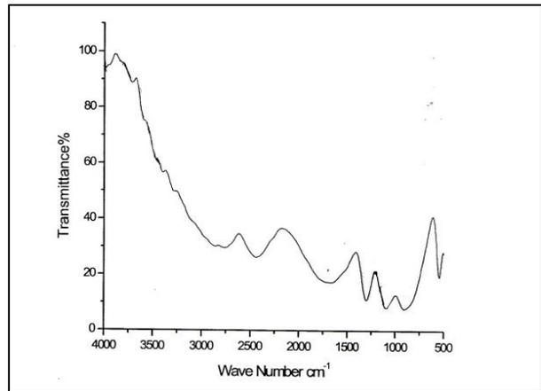
Fig. 3: FTIR Spectrum of Pure KDP Crystal
