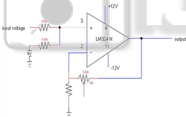
Fig. 4: Signal Conditioning Circuit 2
