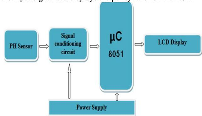
Fig. 1: Block Diagram of Water Purity Indicator
