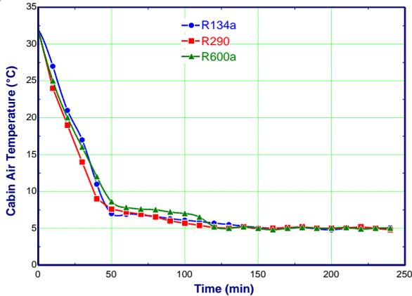
Fig. 10: Pull Down Time Vs. Cabin Air Temperature At 32 °C Ambient Temperature
