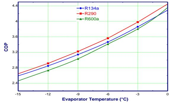
Fig. 7: Experimental COP Comparison
