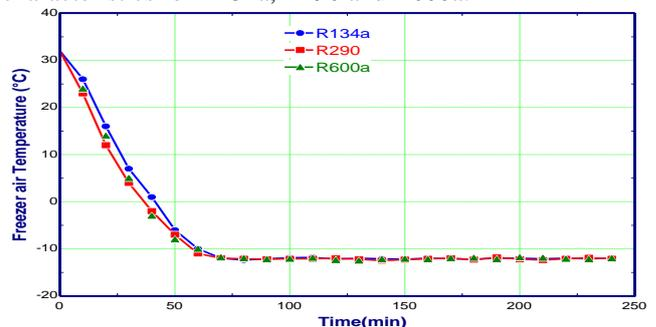
Fig. 9: Pull Down Time Vs. Freezer Air Temperature At 32 °C Ambient Temperature
