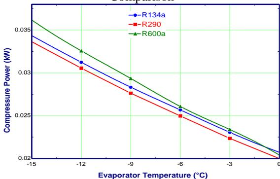
Fig. 6: Experimental Compressor Power Comparison
