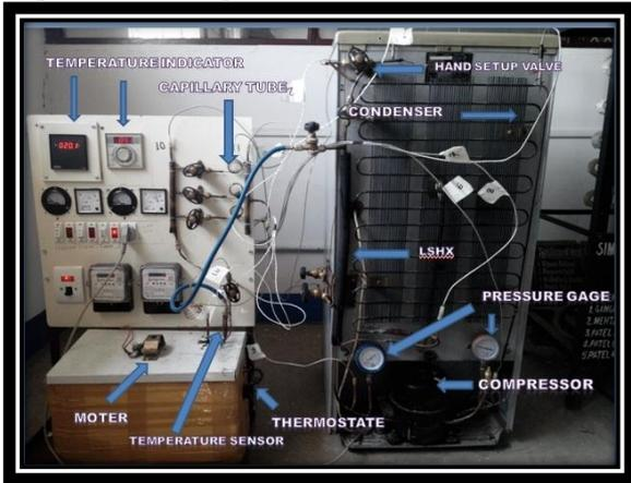
Fig. 4: Experimental Setup
