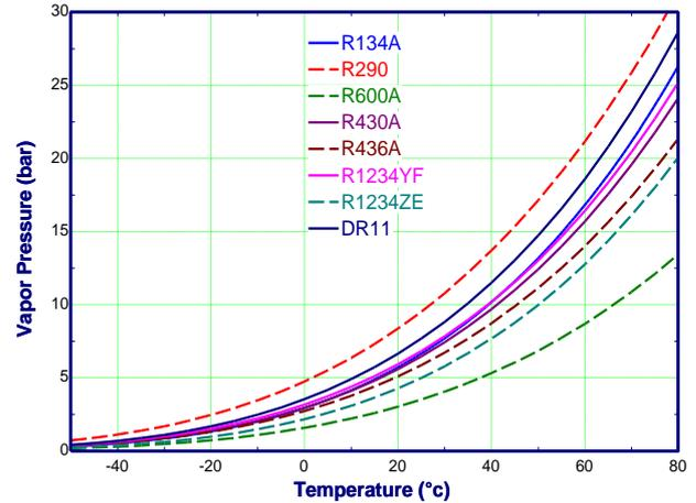
Fig. 1: Variation of Saturation Pressure with Temperature
