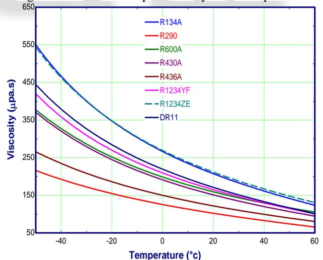
Fig. 3: Liquid viscosity Vs Temperature
