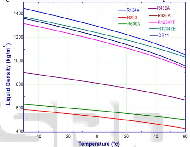
Fig. 2: Variation of Liquid Density with Temperature
