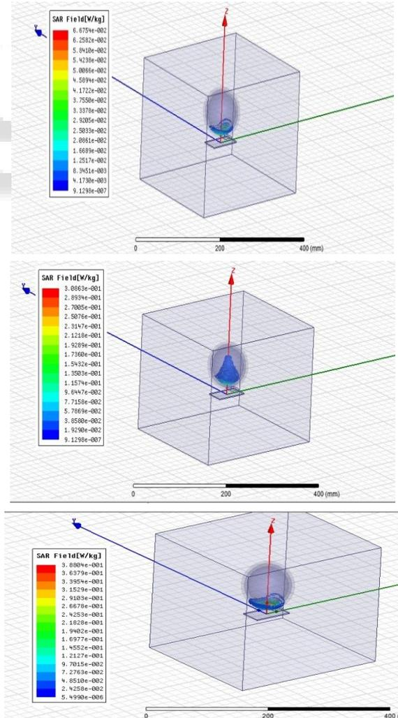
Fig. 5: SAR on 3 layered spherical model, with different tissue bone, brain and skin
