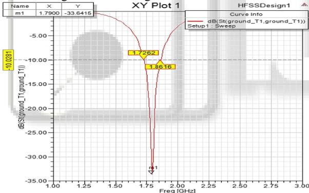
Fig. 5: Return loss of PIFA antenna
