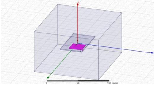
Fig. 3: PIFA design in HFSS at 1.8 GHz
