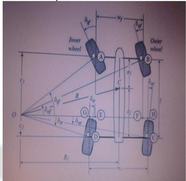
Fig. 2: Steering angles position of Instantaneous center for turning radius 4.4m. [6]
