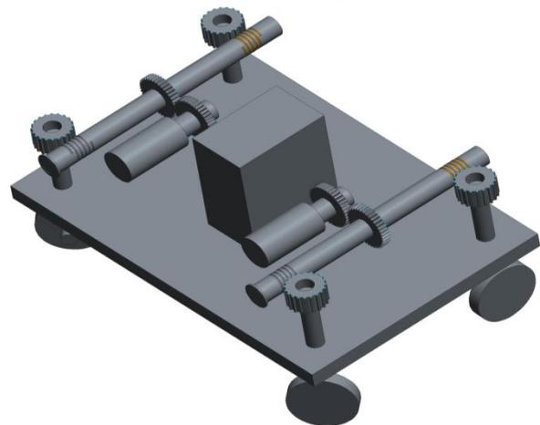
Fig. 3: CAD Model of 90 Degree Turning Car
