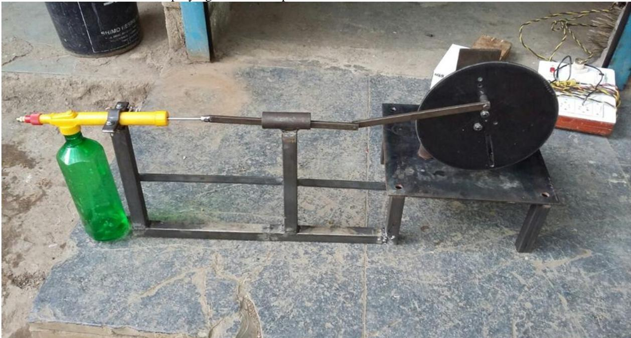
Fig. 1: Crank and Lever Reciprocating Mechanism
