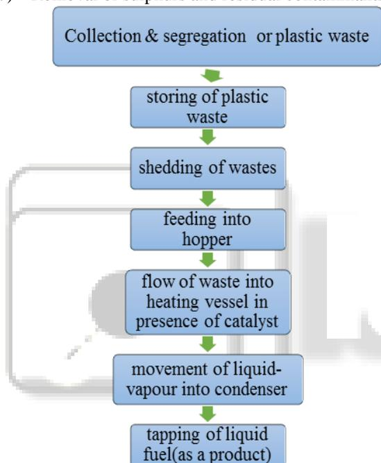
Fig. 2: Conversion of Plastics waste into Liquid Fuel
