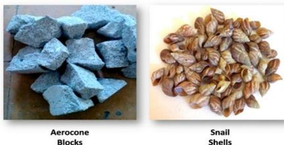
Fig. 1: Media/Materials used in Customized Constructed Wetland
