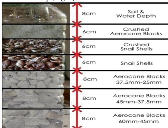
Fig. 2: Arrangement of Different Size of Media
