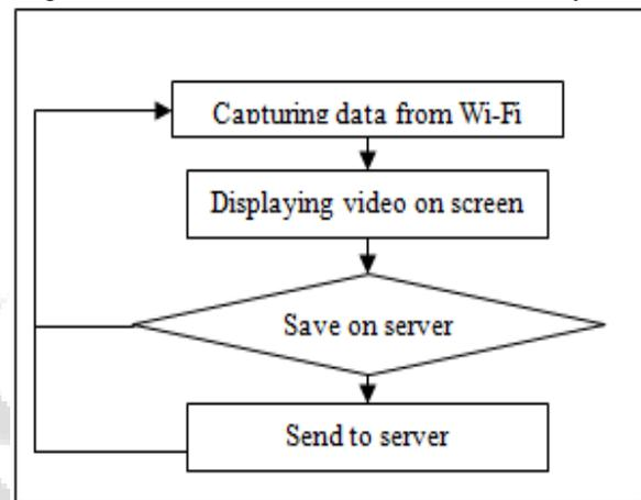
Fig. 3: Flow chart of receiving software system
