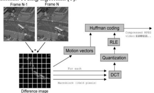
Fig. 6: Flow of MPEG-2 Compression Algorithm
