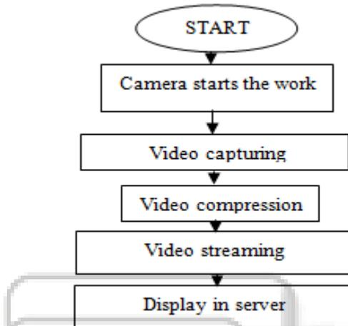
Fig. 5: Flow Chart of Software System [1]
