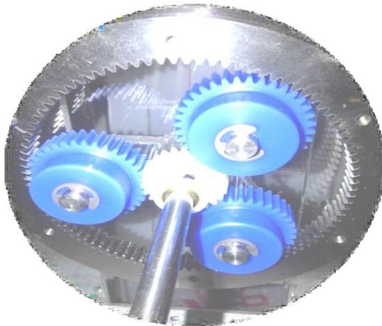
Fig. 1: 3D view of Planetary
