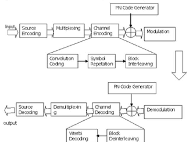
Fig 1. Block diagram of the CDMA technology
