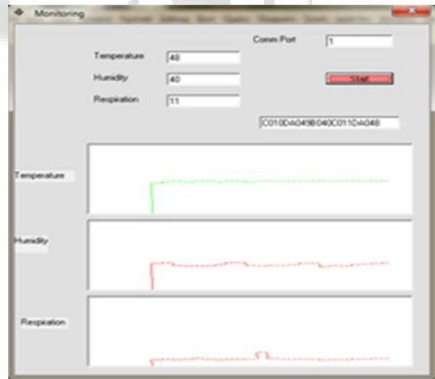
Fig. 6: Visual basic output of Temperature, Humidity and Respiration.
