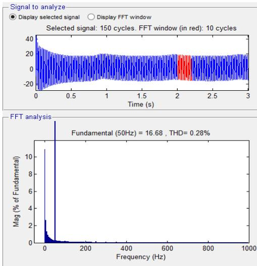
Fig. 5: Current THD for compensated system using BP
