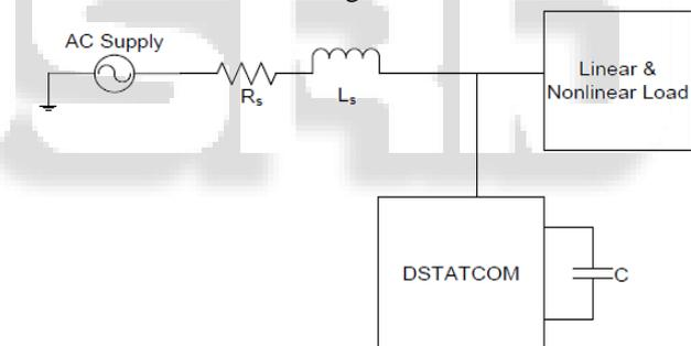
Fig. 1: Basic building blocks of DSTATCOM
