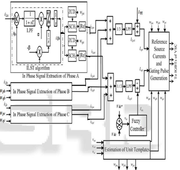
Fig. 3: Generation of reference source currents using ILST control algorithm
