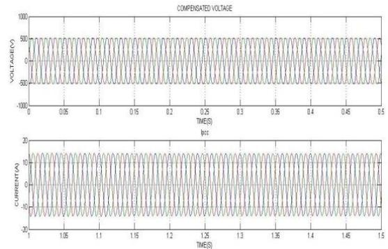
Fig. 8: Compensated output voltage and current waveforms using ILST algorithm
