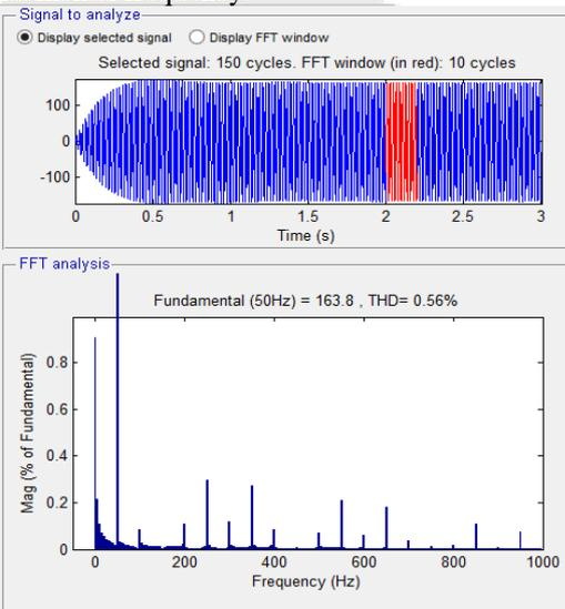
Fig. 6: Voltage THD for compensated system using BP
