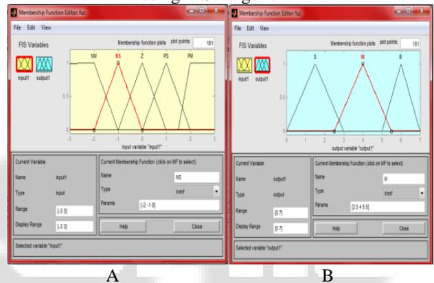
Fig. 9: Input and Output variables in Fuzzy controller for ILST Algorithm
