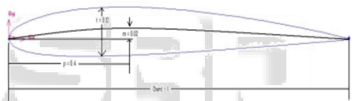
Fig. 9: Diagram displaying the chord length, maximum chamber, position of max chamber and max thickness of the airfoil geometry
