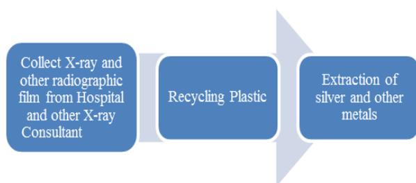
Fig. 5: Methodology for Recycle Photographic film
