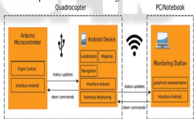
Fig. 6: Software modules of the proposed setup.
