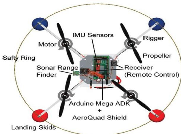
Fig. 5: All hardware components of the UAV.
