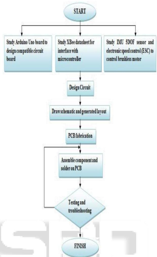
Fig. 3: Quadcopter Design Flowchart
