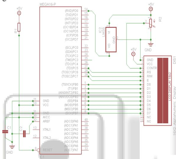
Fig. 2: Circuit Diagram of Temperature Sensor
