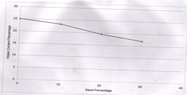
Fig. 4(a): plastic limit of Yellow soil mixed with sand grade-II
