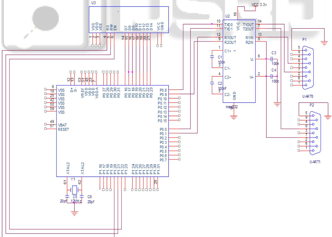
Fig. 4: Circuit diagram of server unit
