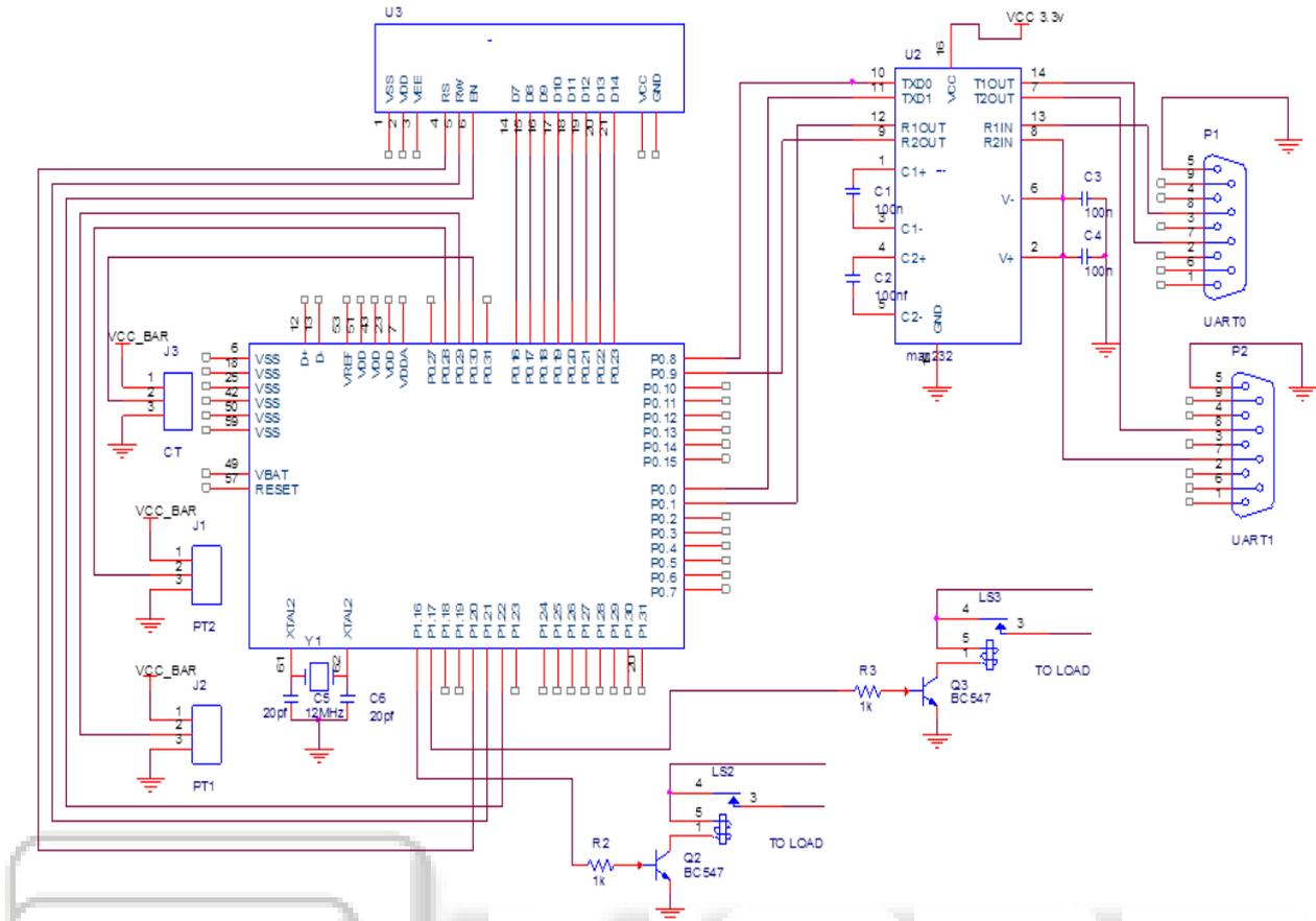
Fig. 3: Circuit diagram of consumer unit
