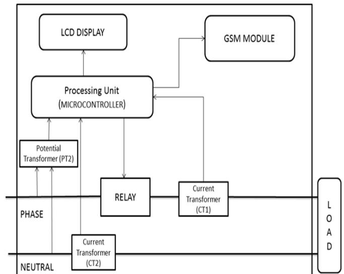
Fig. 2: Block diagram of consumer unit
