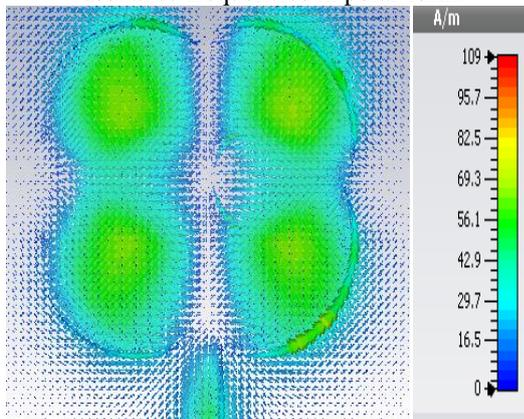
Fig. 7: Surface Current distribution profile of proposed antenna at 7.2GHz, 9.2GHz, 10GHz and 11.7GHz
