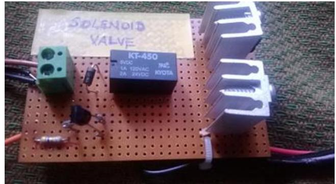
Fig. 2.2: Driver circuit
