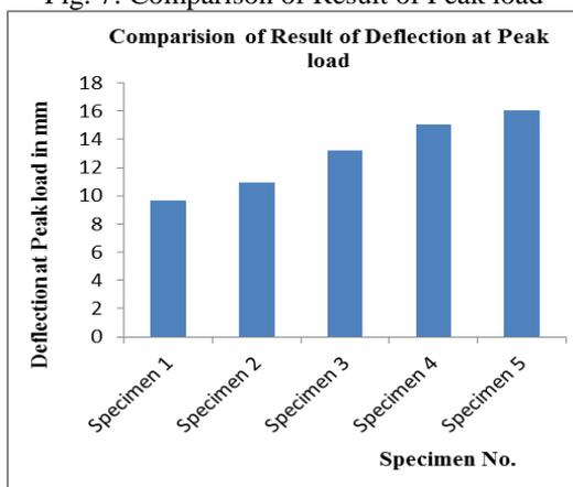
Fig. 8: Comparison of Result of Deflection at Peak load
