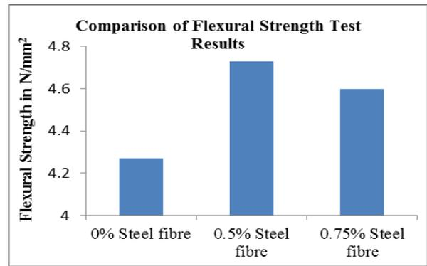
Fig. 3: Comparison of Flexural Strength Test Result
