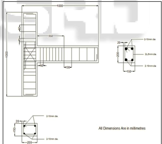
Fig. 4: Reinforcement details as per I.S. 13920:1993 and diagonal cross inclined bar
