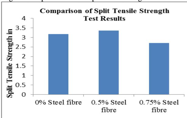
Fig. 2: Comparison of Split Tensile Strength Test Result
