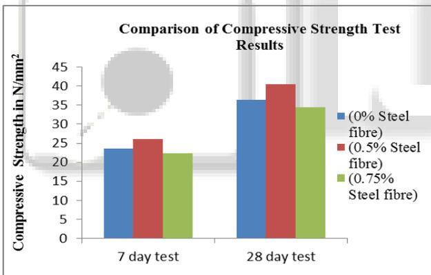
Fig. 1: Comparison of Compressive Strength Test Result
