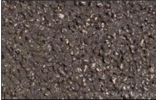
Fig. 3: Open graded HMA
