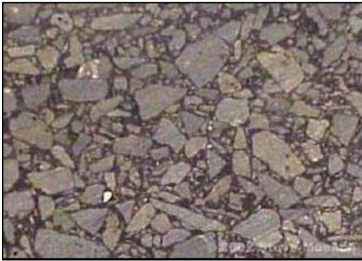
Fig. 2: Dense graded HMA
