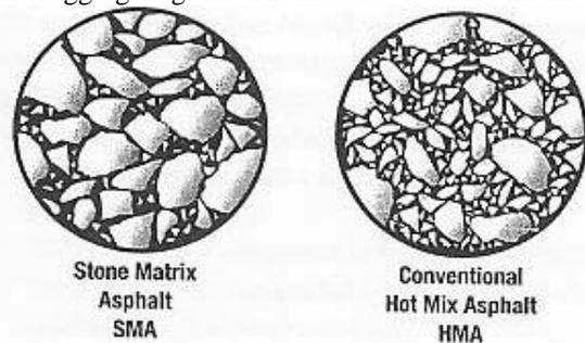
Fig. 1: comparison between SMA and conventional HMA
